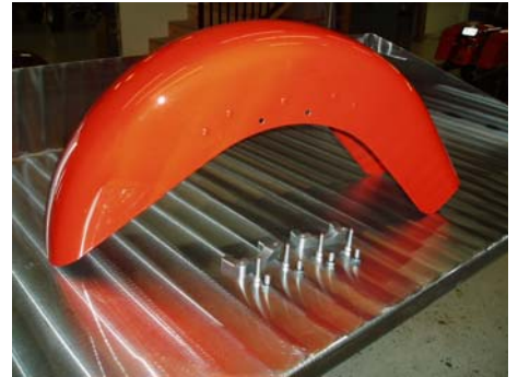
Figure 17 – Fender ready for new brackets
